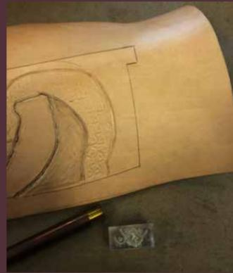
To create the file to be 3d printed the scale pattern was drafted through tinker cad. I first thought the stamp would be more efficient if the scales were in a cluster of four. The draft was printed with a resin printer which creates the shape by pulling it out of a bath of melted plastic. However once doing a sample (as seen on the right) the stamp worked but I realized that the cluster method would not work with the scale of my pattern pieces and design.
