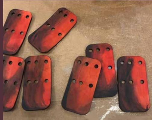
I cut 2 sets of 56 tiles equaling 112, and then used scraps to cut approximately 40 more. The laser cutting process took about 2.5 hours total with no stress on my hands.
