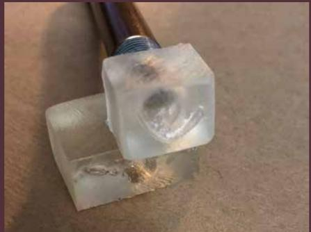
The pictures to the bottom left show the changes that were made after the first attempt. I simplified the file to just be one scale and adjusted the hole in the bottom to be the correct size. In my first attempt I also realized that the height of the scale pattern was a problem because it would just keep cracking and I would have to keep filing it down, so that was adjusted.
