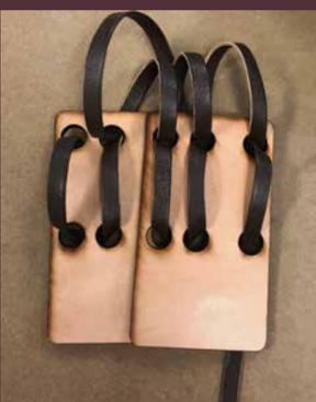
When starting this project the idea of hand cutting all of the tiles in the skirt portion of the armor was out of question. The idea of laser cutting was the solution. For my first sample of how it would work I cut just a couple tiles to get an idea of how it could work along with how to do the lacing. I discovered that my tiles were too wide, my corners to sharp, and the holes too big.
